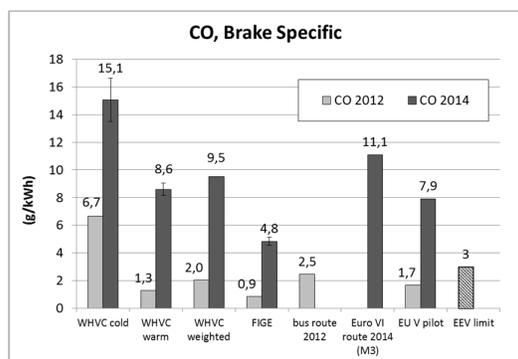
Figure 8 Brake specific CO emissions.
