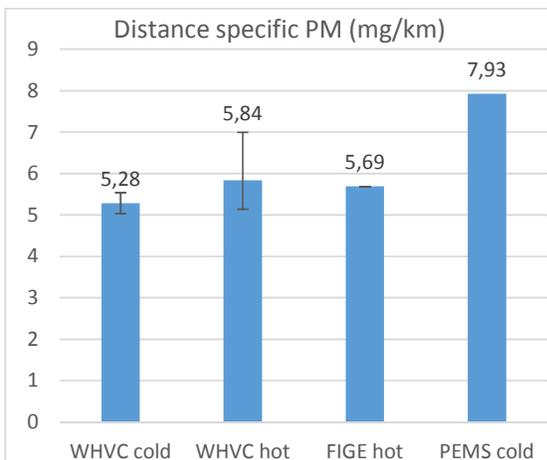
Figure 108. Avg. dist. specific PM emissions (mg/km)
