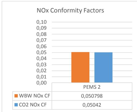
Figure 162. NOx Conformity factors for the normal PEMS test using work based windows (WBW) and CO<sub>2</sub> mass based windows, respectively.
