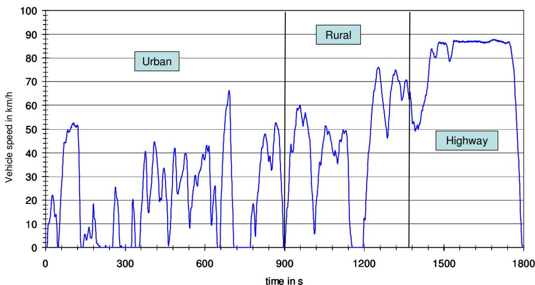
Figure 3 The WHVC test cycle
