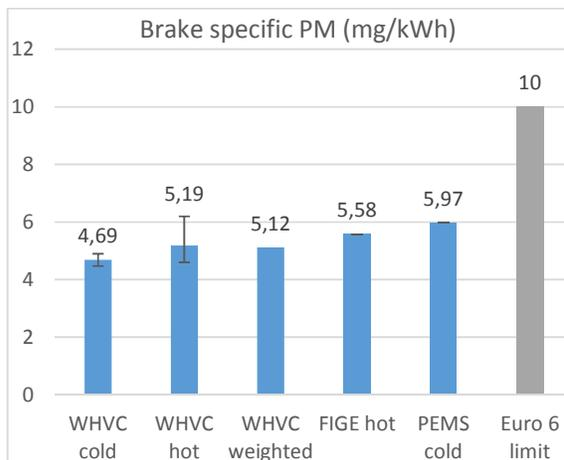
Figure 107. Avg. brake specific PM emissions (mg/kWh)
