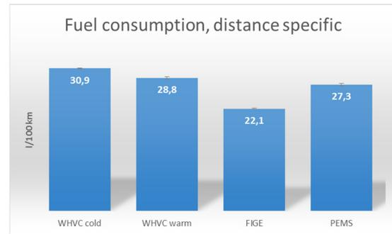
Figure 42 Distance specific fuel consumption
