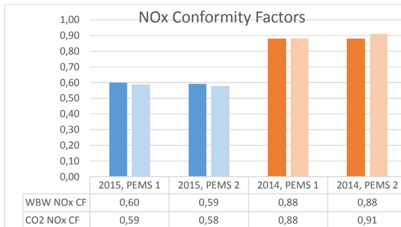
Figure 121. Work and CO<sub>2</sub> based conformity factors for NO<sub>x</sub>.
