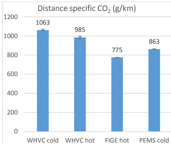
Figure 113. Avg. distance specific CO<sub>2</sub> emissions (g/km)
