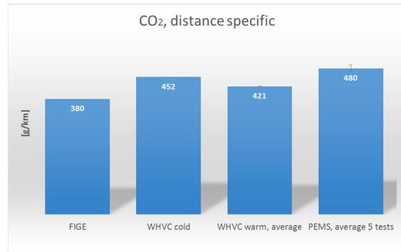
Figure 59 Distance specific CO<sub>2</sub> emissions.
