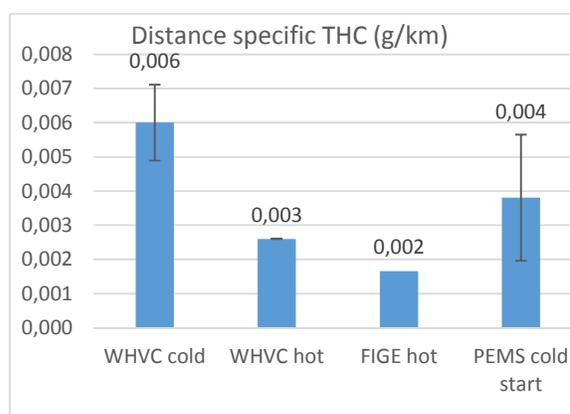
Figure 87 Avg. distance specific THC emissions (g/km)
