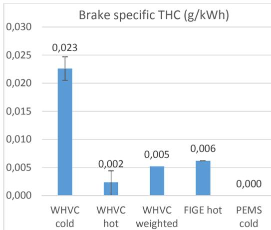
Figure 103. Avg. brake specific THC emissions (g/kWh)
