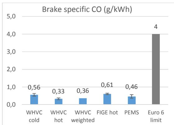
Figure 146. Avg. brake specific CO emissions (g/kWh)
