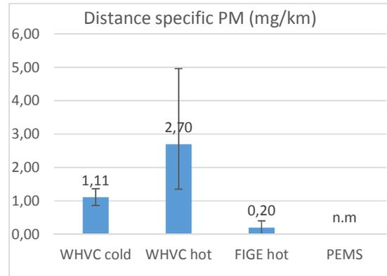
Figure 153. Avg. distance specific PM emissions (g/km)
