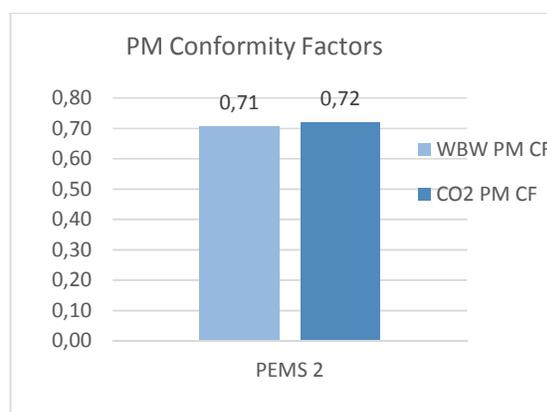
Figure 100. Work and CO<sub>2</sub> based PM conformity factors for the second PEMS test.
