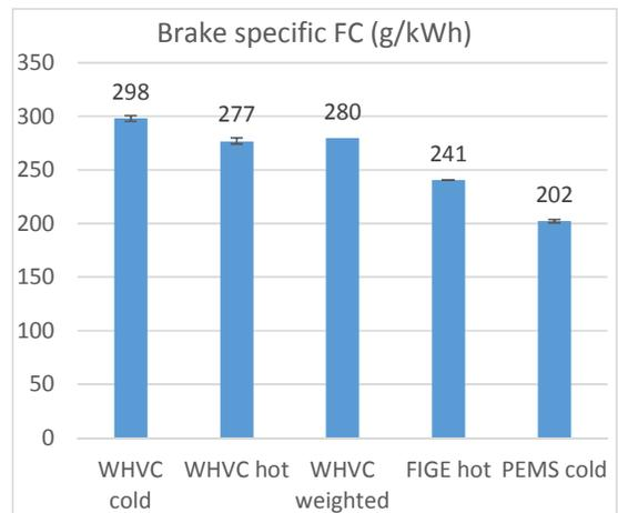
Figure 112. Avg. brake specific FC (g/kWh)
