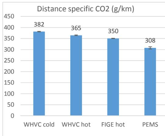
Figure 158. Avg. distance specific CO<sub>2</sub> emissions (g/km)
