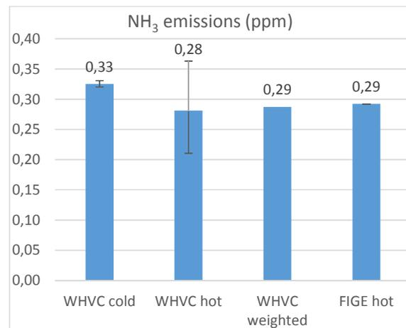
Figure 116. Avg. NH<sub>3</sub> emissions over chassis dynamometer tests (ppm)
