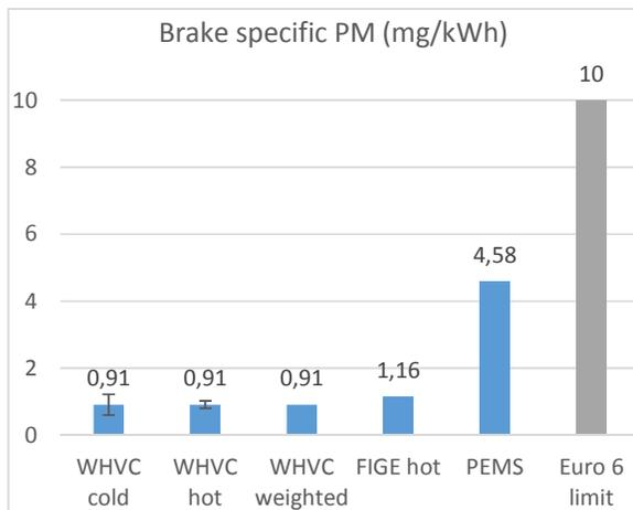
Figure 133. Avg. brake specific PM emissions (g/kWh)
