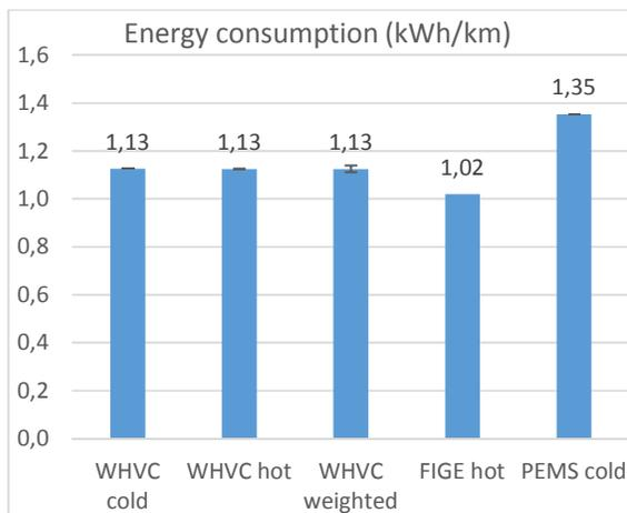
Figure 115. Avg. energy consumption (kWh/km)
