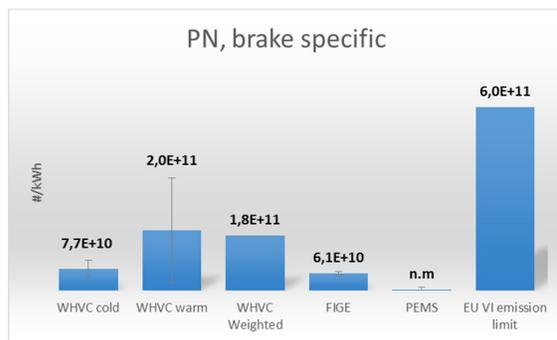
Figure 37 Brake specific PN emissions.
