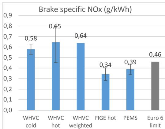
Figure 150. Avg. brake specific NO<sub>x</sub> emissions (g/kWh)
