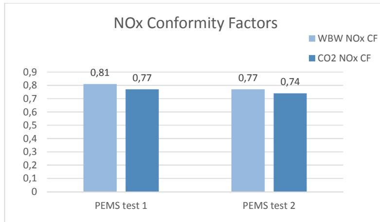
Figure 126. NO<sub>x</sub> Conformity factors for the PEMS tests using work based windows (WBW) and CO<sub>2</sub> mass based windows, respectively.
