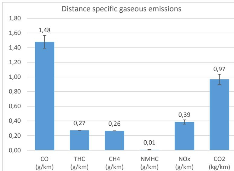
Figure 119. Avg. distance specific gaseous emissions.
