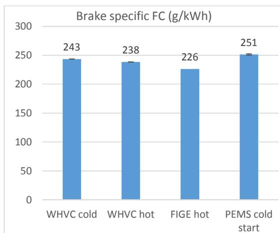
Figure 96 Avg. brake specific FC (g/kWh)
