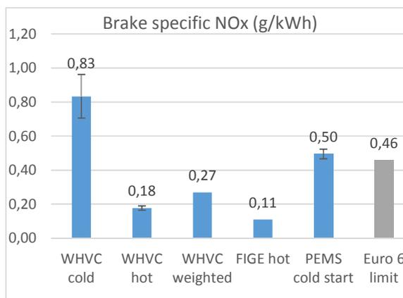
Figure 88 Avg. brake specific NO<sub>x</sub> emissions (g/kWh)
