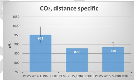
Figure 24 Distance specific CO<sub>2</sub> emissions.
