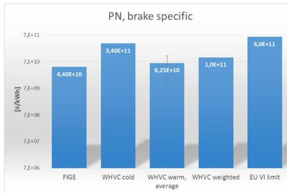
Figure 56 Brake specific PN emissions.
