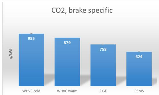
Figure 39 Brake specific CO<sub>2</sub> emissions.
