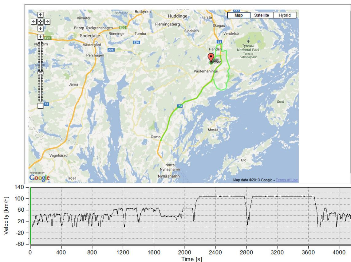
Figure 7 Characteristics of the PEMS Pilot route
