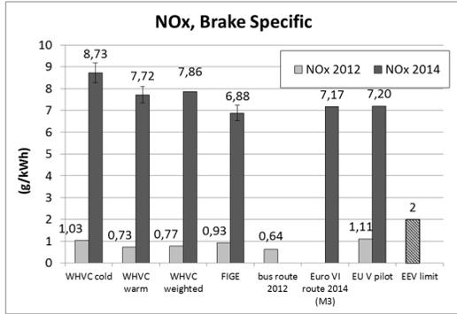
Figure 12 Brake specific NOx emissions.
