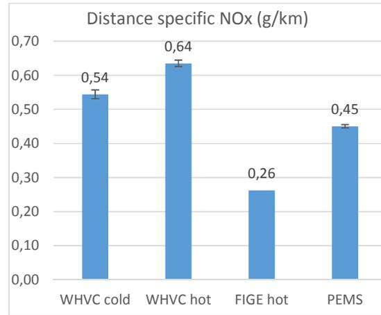
Figure 132. Avg. distance specific NO<sub>x</sub> emissions (g/km)
