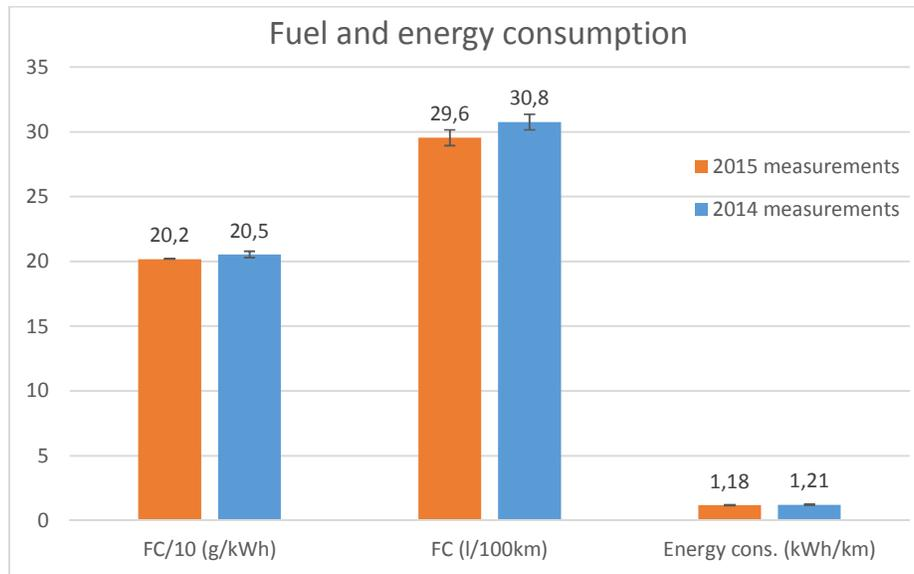
Figure 125. Avg. brake and distance specific fuel consumption and energy consumption.
