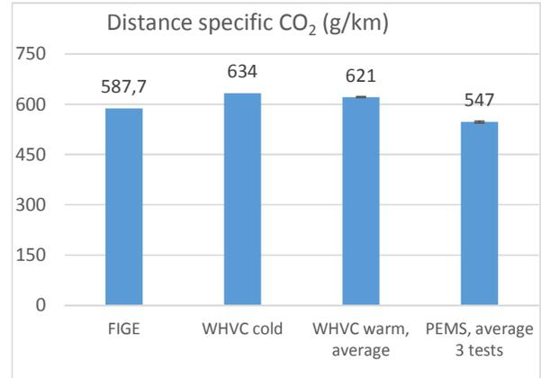
Figure 75. Distance specific CO<sub>2</sub> emissions.
