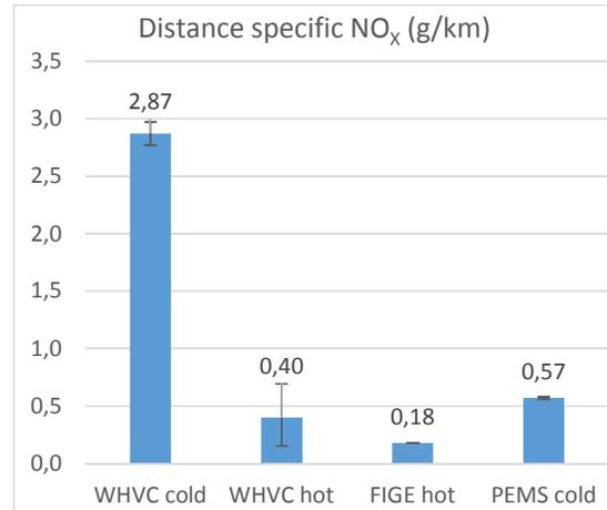
Figure 106. Avg. distance specific NO<sub>x</sub> emissions (g/km)
