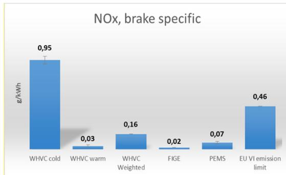
Figure 32 Brake specific NOx emissions.
