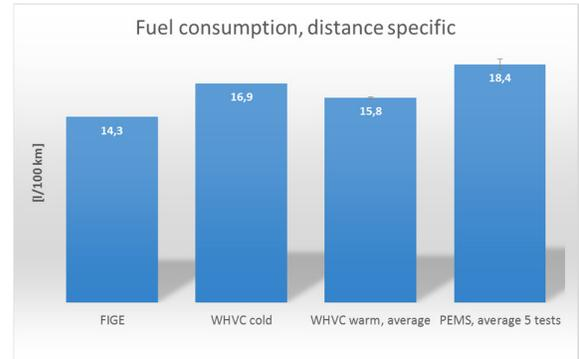
Figure 61 Distance specific fuel consumption
