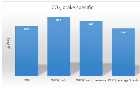
Figure 58 Brake specific CO<sub>2</sub> emissions.
