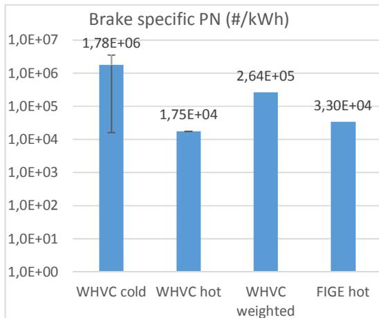
Figure 135. Avg. brake specific PN emissions (#/kWh)
