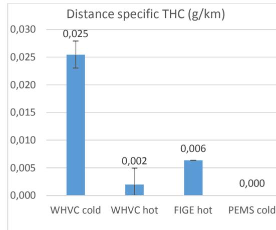
Figure 104. Avg. distance specific THC emissions (g/km)
