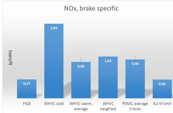
Figure 50 Brake specific NOx emissions.
