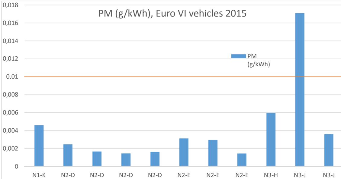
Figure 1724. PM emissions from 2015 testing
