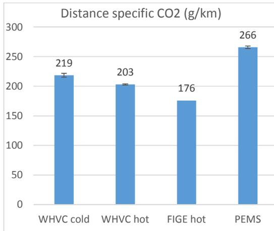
Figure 139. Avg. distance specific CO2 emissions (g/km')
