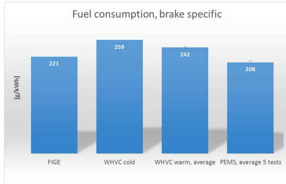
Figure 60 Brake specific fuel consumption.
