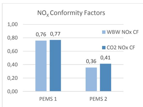
Figure 99. Work and CO<sub>2</sub> based NO<sub>x</sub> conformity factors for both PEMS tests.
