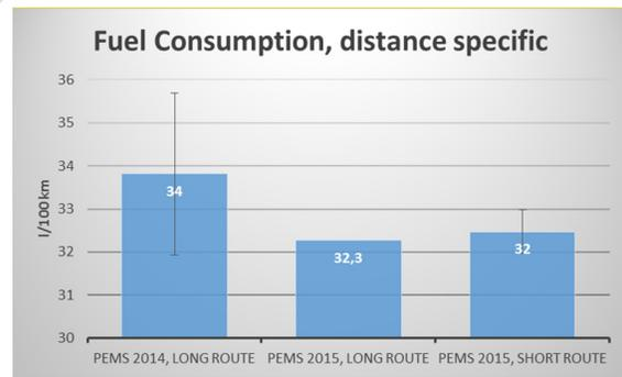
Figure 26 Distance specific fuel consumption
