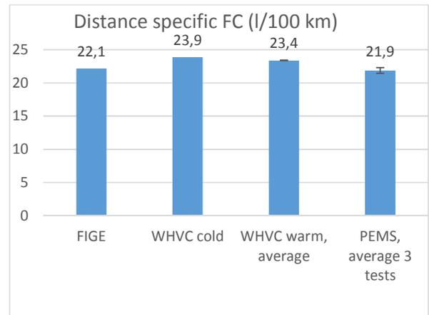
Figure 77 Distance specific fuel consumption
