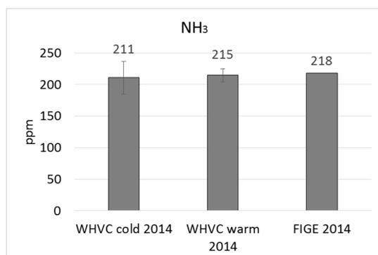
Figure 19 Emissions of ammonia (average ppm level)
