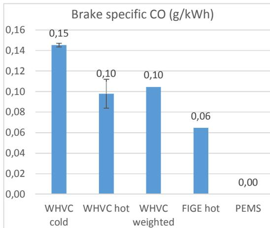
Figure 127. Avg. brake specific CO emissions (g/kWh)
