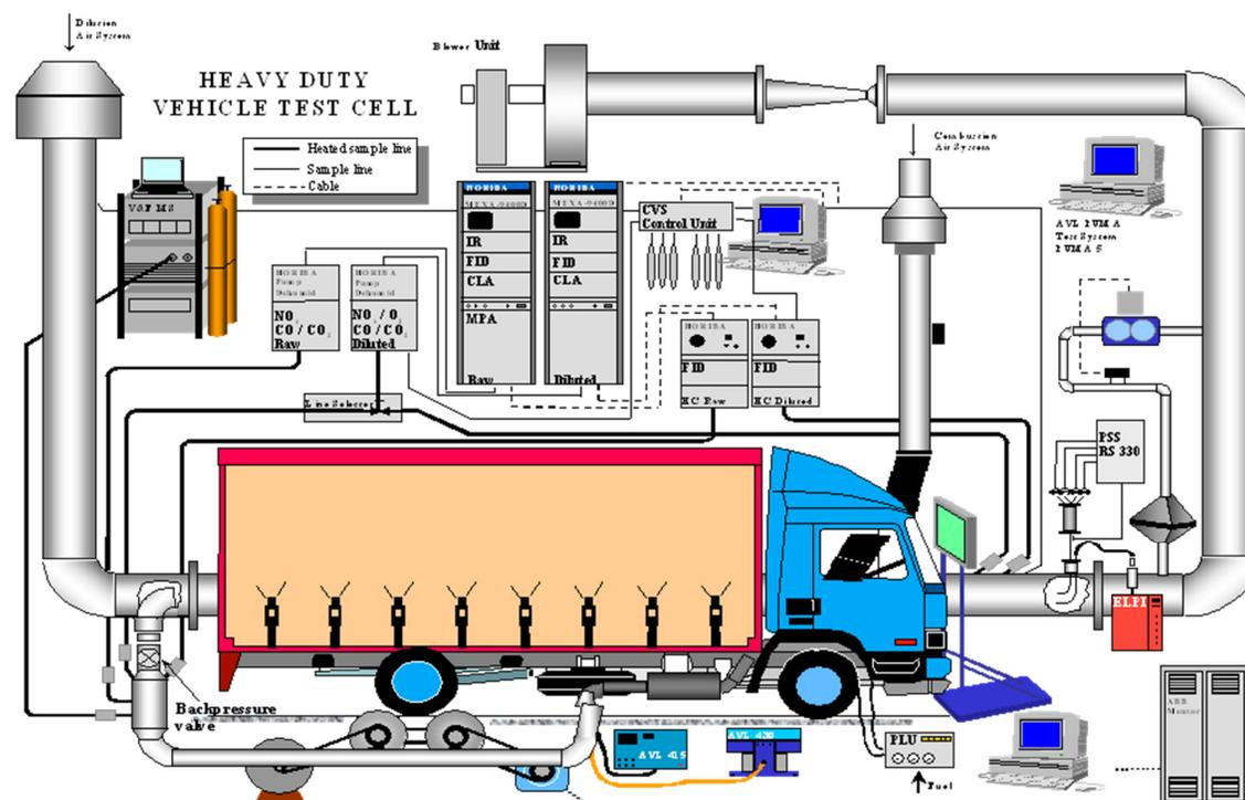
Figure 1 A schematic description of the test cell.
