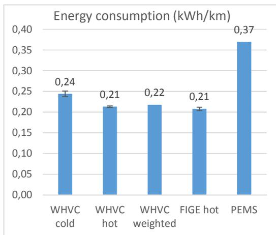
Figure 141. Avg. energy consumption (kWh/km)
