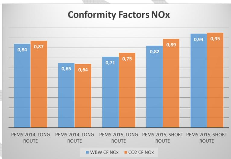
Figure 20 Conformity Factors for NO<sub>x</sub>
