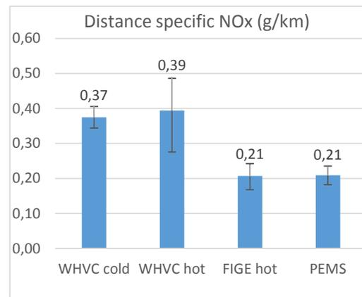
Figure 151. Avg. distance specific NO<sub>x</sub> emissions (g/km)
