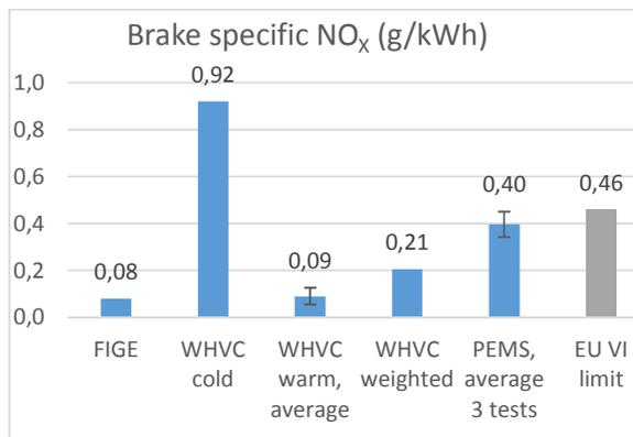
Figure 67. Brake specific NO<sub>x</sub> emissions.
