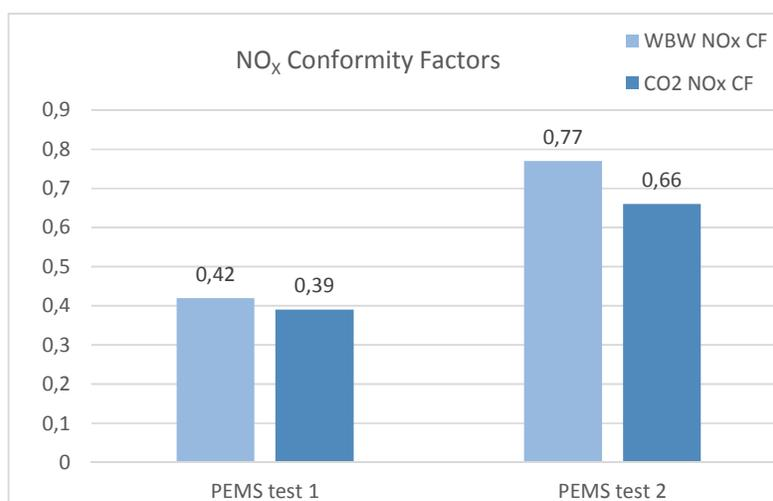
Figure 83. NO<sub>x</sub> Conformity factors for the PEMS tests using the Work based windows (WBW) and CO<sub>2</sub> mass based windows, respectively.
