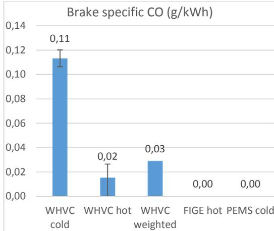
Figure 101. Avg. brake specific CO emissions (g/kWh)
