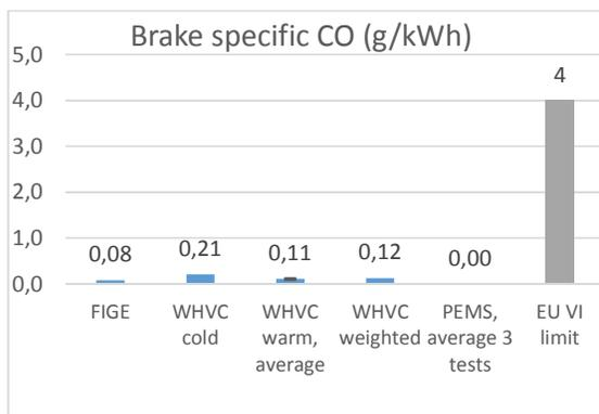
Figure 65. Brake specific CO emissions.
