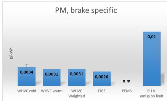
Figure 35 Brake specific PM emissions.
