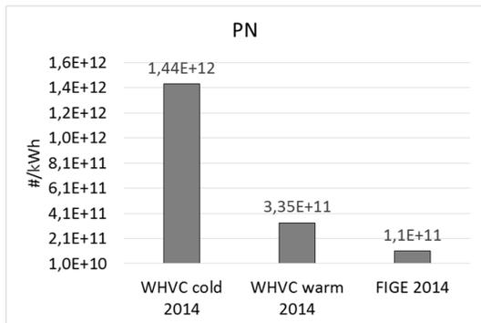
Figure 16 Brake specific PN emissions.
