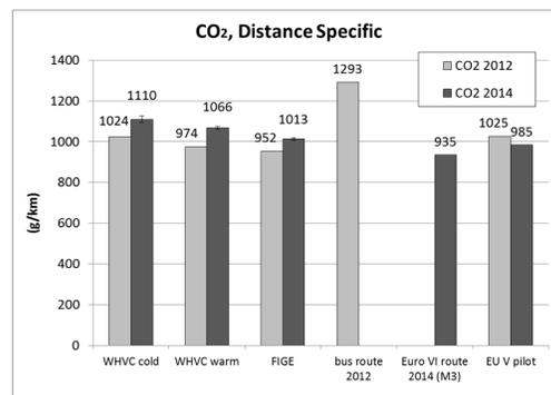
Figure 18 Distance specific CO<sub>2</sub> emissions
