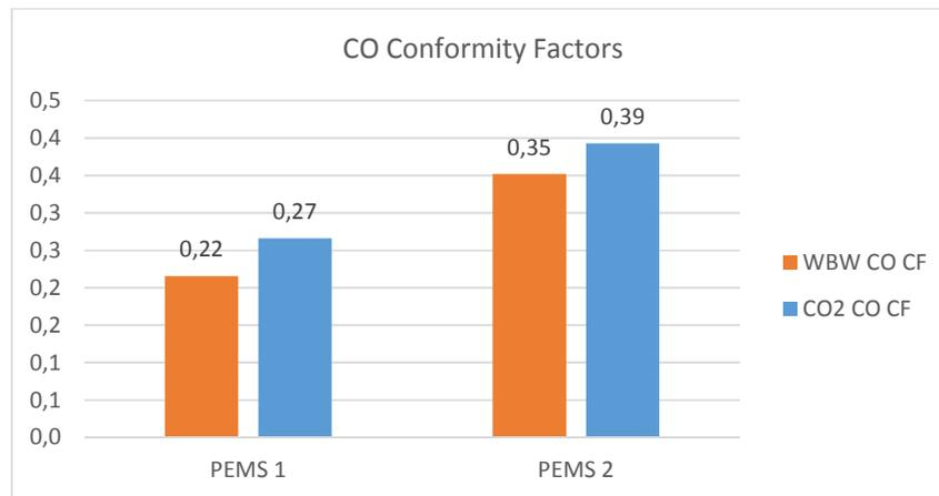
Figure 143 CO Conformity factors for the PEMS tests using work based windows (WBW) and CO<sub>2</sub> mass based windows, respectively.
