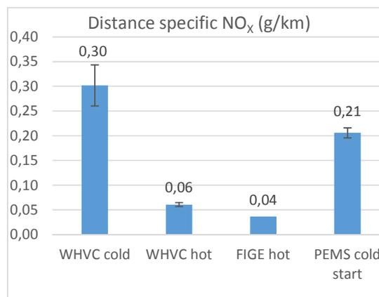
Figure 89 Avg. distance specific NO<sub>x</sub> emissions (g/km)
