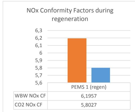
Figure 163 NOx Conformity factors for the PEMS test when DPF regeneration occurred, using work based windows (WBW) and CO<sub>2</sub> mass based windows, respectively.
