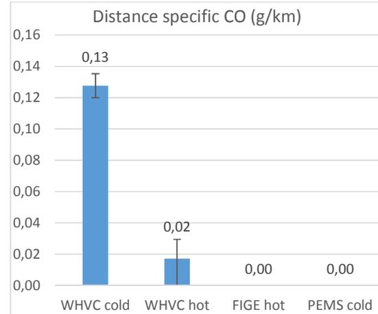
Figure 102. Avg. distance specific CO emissions (g/km)
