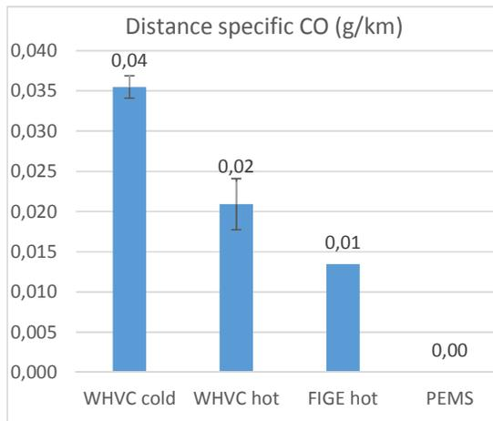
Figure 128. Avg. distance specific CO emissions (g/km)
