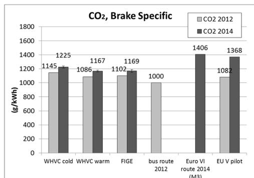
Figure 17 Brake specific CO<sub>2</sub> emissions.
