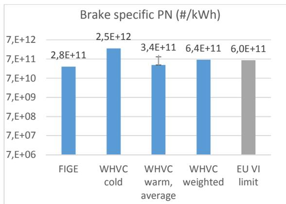
Figure 72. Brake specific PN emissions.
