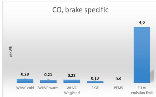
Figure 30 Brake specific CO emissions.
