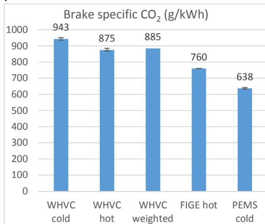
Figure 111. Avg. brake specific CO<sub>2</sub> emissions (g/kWh)
