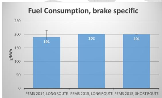
Figure 25 Brake specific fuel consumption.
