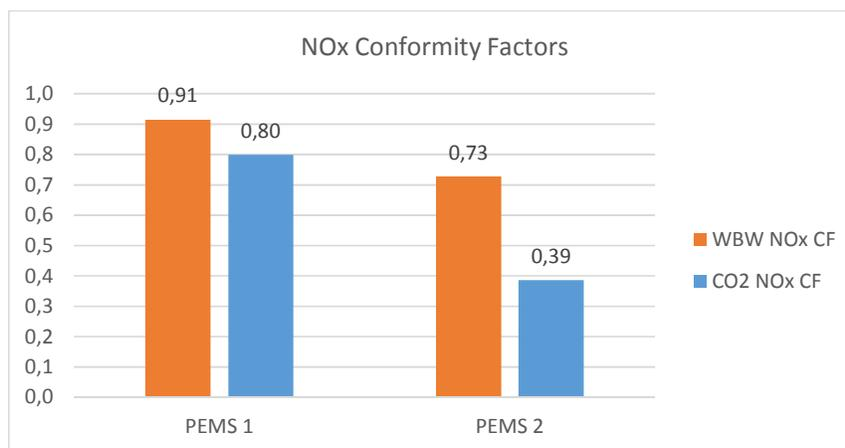
Figure 144. NOx Conformity factors for the PEMS tests using work based windows (WBW) and CO<sub>2</sub> mass based windows, respectively.
