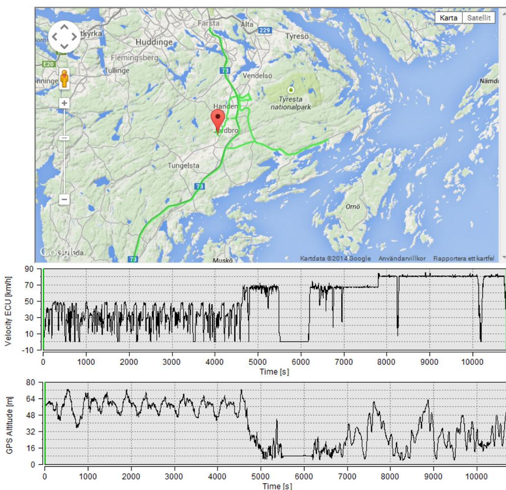
Figure 5 Characteristics of the Euro VI route for N1, N2, M1, M2 and M3 vehicles
