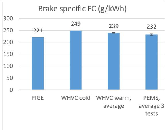
Figure 76. Brake specific fuel consumption.
