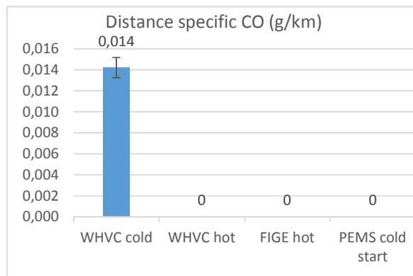
Figure 85 Avg. distance specific CO emissions (g/km)
