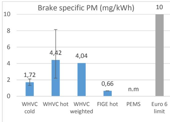
Figure 152. Avg. brake specific PM emissions (g/kWh)
