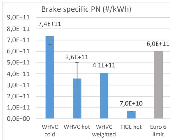
Figure 154. Avg. brake specific PN emissions (#/kWh)
