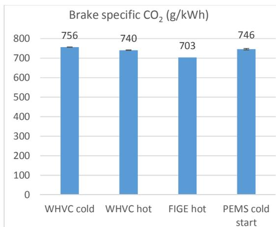
Figure 94 Avg. brake specific CO<sub>2</sub> emissions (g/kWh)
