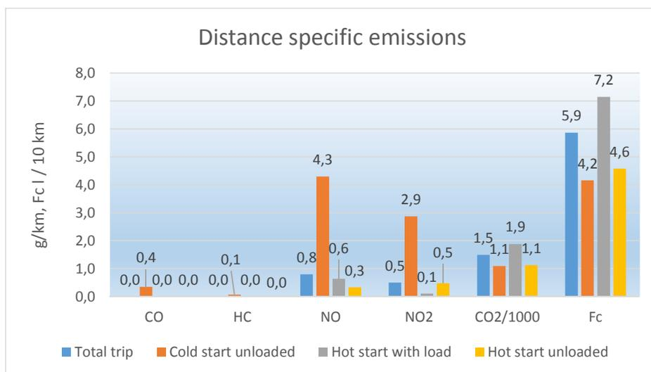
Figure 81 Distance specific emissions for the complete test and sub trips.
