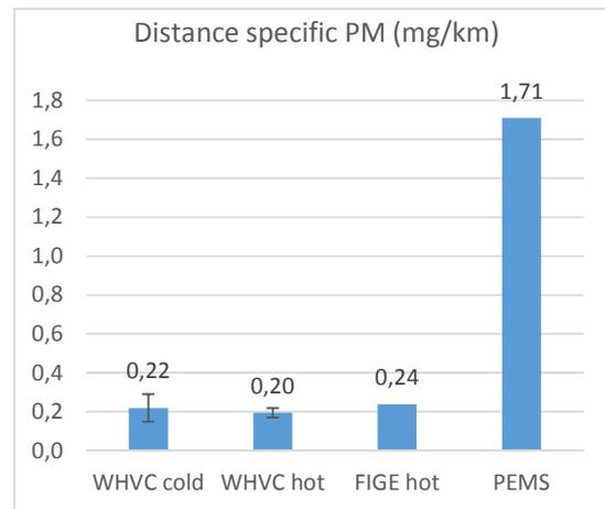
Figure 134. Avg. distance specific PM emissions (g/km)
