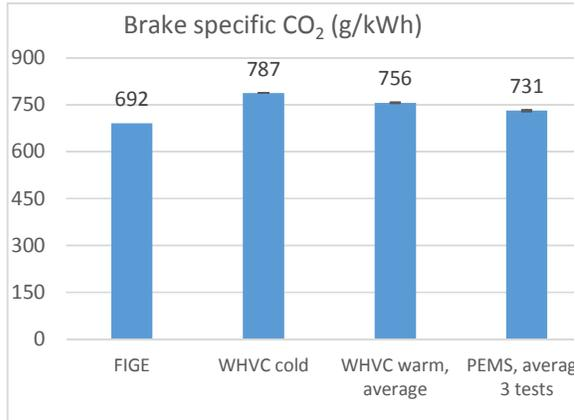
Figure 74. Brake specific CO<sub>2</sub> emissions.
