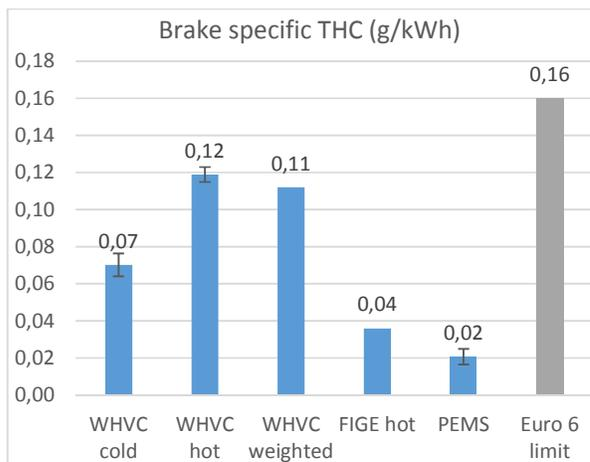
Figure 129. Avg. brake specific THC emissions (g/kWh)
