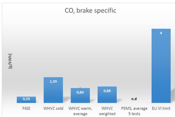
Figure 48 Brake specific CO emissions.
