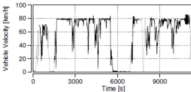
Figure 79 Test trip driving pattern.
