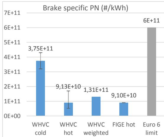
Figure 109. Avg. brake specific PN emissions (#/kWh)
