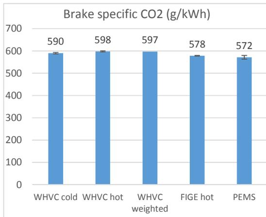
Figure 156. Avg. brake specific CO<sub>2</sub> emissions (g/kWh)
