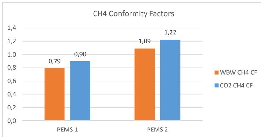
Figure 145 CH4 Conformity factors for the PEMS tests using work based windows (WBW) and CO2 mass based windows, respectively.
