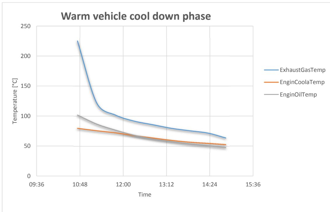
Figure 28 Cool down phase of warm vehicle
