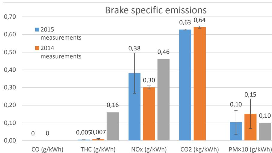
Figure 123. Avg. brake specific emissions.
