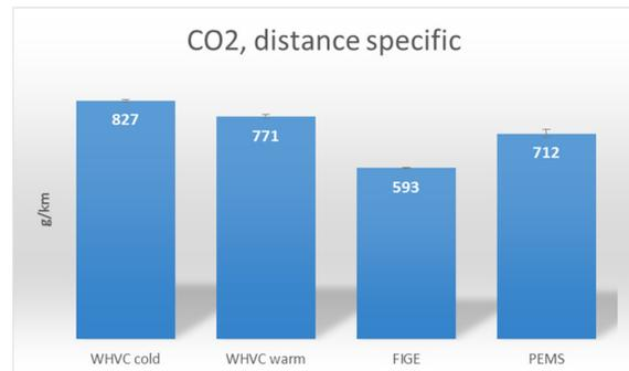
Figure 40 Distance specific CO<sub>2</sub> emissions.
