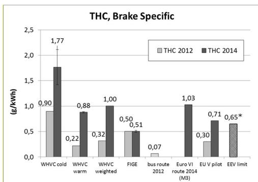
Figure 10 Brake specific THC emissions.
