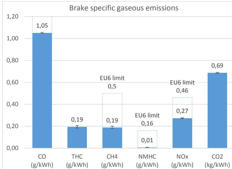
Figure 118. Avg. brake specific gaseous emissions.
