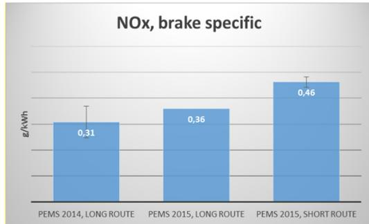
Figure 21 Brake specific NOx emissions.
