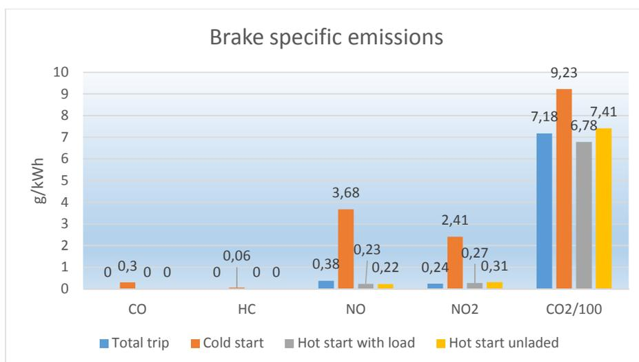
Figure 80 Brake specific emissions for the complete test and sub trips.
