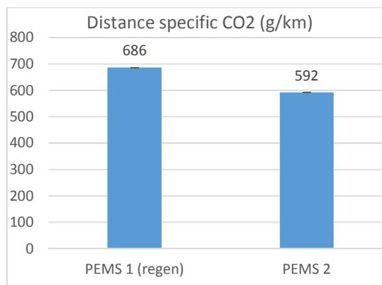
Figure 168. Avg. distance specific CO<sub>2</sub> emissions (g/km)
