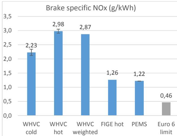
Figure 131. Avg. brake specific NO<sub>x</sub> emissions (g/kWh)
