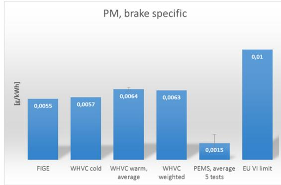
Figure 54 Brake specific PM emissions.
