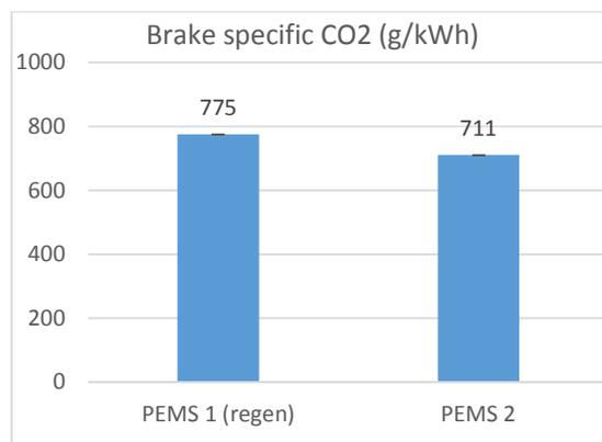
Figure 166. Avg. brake specific CO<sub>2</sub> emissions (g/kWh)
