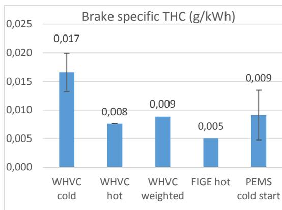
Figure 86 Avg. brake specific THC emissions (g/kWh)
