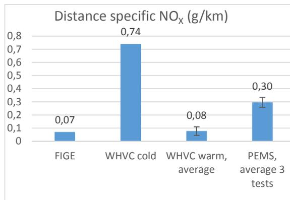
Figure 68 Distance specific NO<sub>x</sub> emissions.
