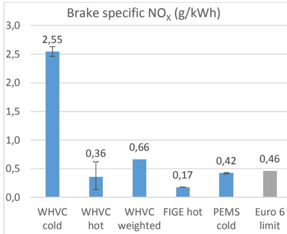
Figure 105. Avg. brake specific NO<sub>x</sub> emissions (g/kWh)
