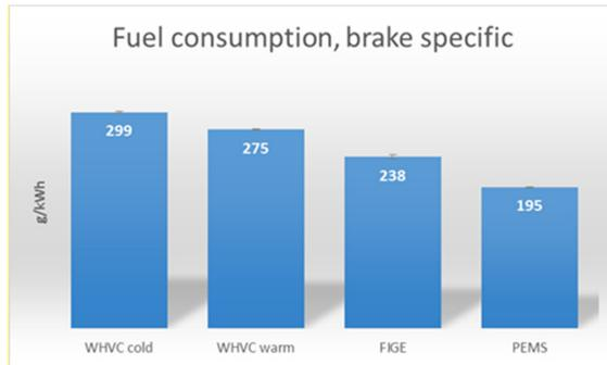
Figure 41 Brake specific fuel consumption.
