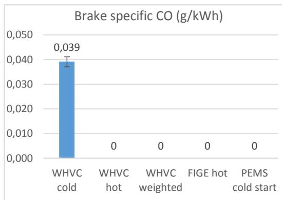
Figure 84 Avg. brake specific CO emissions (g/kWh)
