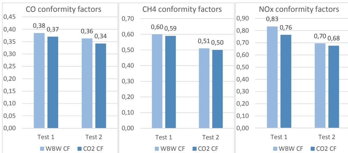
Figure 117. Work and CO<sub>2</sub> based conformity factors for CO, CH<sub>4</sub> and NO<sub>x</sub> from PEMS trip 1 and 2.
