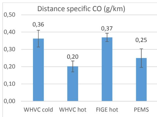
Figure 147. Avg. distance specific CO emissions (g/km)
