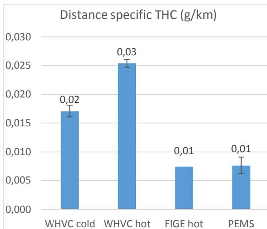
Figure 130. Avg. distance specific THC emissions (g/km)
