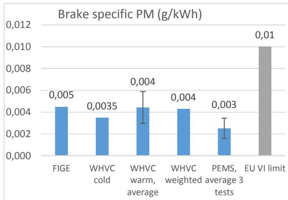
Figure 70. Brake specific PM emissions.
