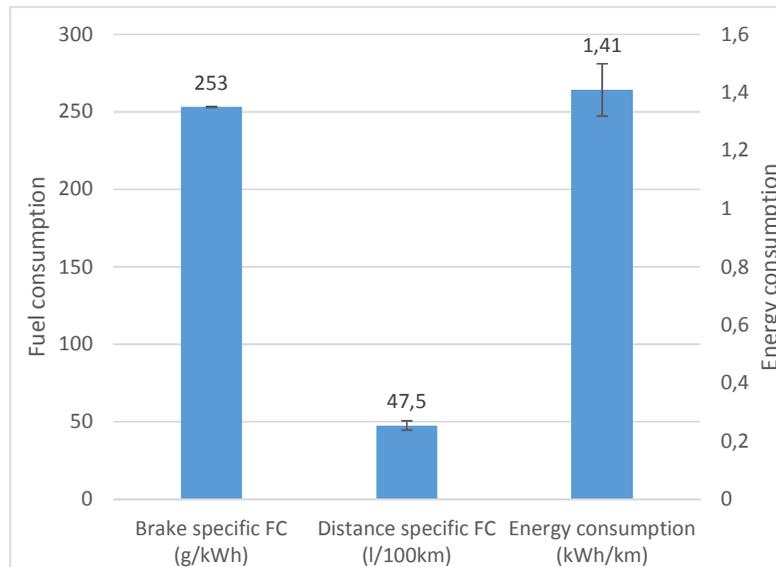
Figure 120. Avg. brake and distance specific fuel consumption and energy consumption.
