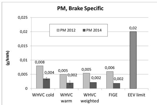
Figure 14 Brake specific PM emissions.
