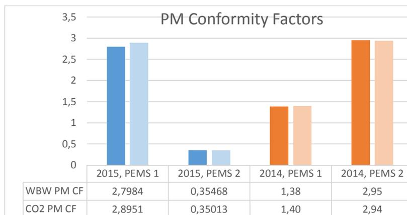
Figure 122. Work and CO<sub>2</sub> based conformity factors for PM.
