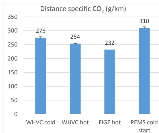
Figure 95 Avg. distance specific CO<sub>2</sub> emissions (g/km)
