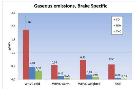
Figure 9 Brake specific gaseous emissions
