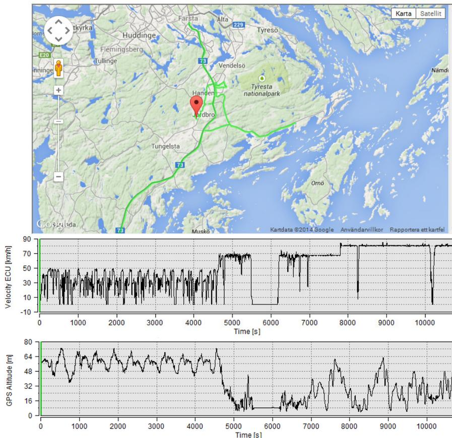
Figure 7 Map showing the EuroVI route 3. The red mark indicates the starting point. The diagram below the map shows the terrain profile and typical vehicle velocities.
