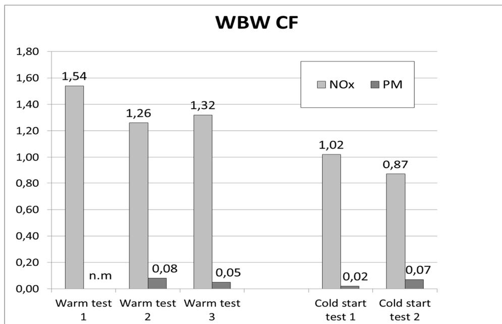
Figure 50 Work based windows, NOx and PM conformity factors
