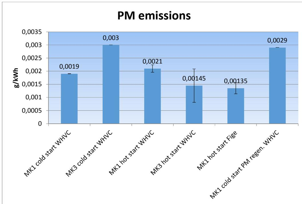
Figure 121 Particle mass emissions g/kWh.
