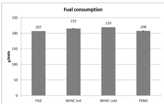
Figure 28 Brake specific fuel consumption.
