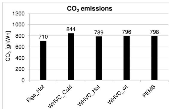
Figure 107 Brake specific CO<sub>2</sub> emissions.
