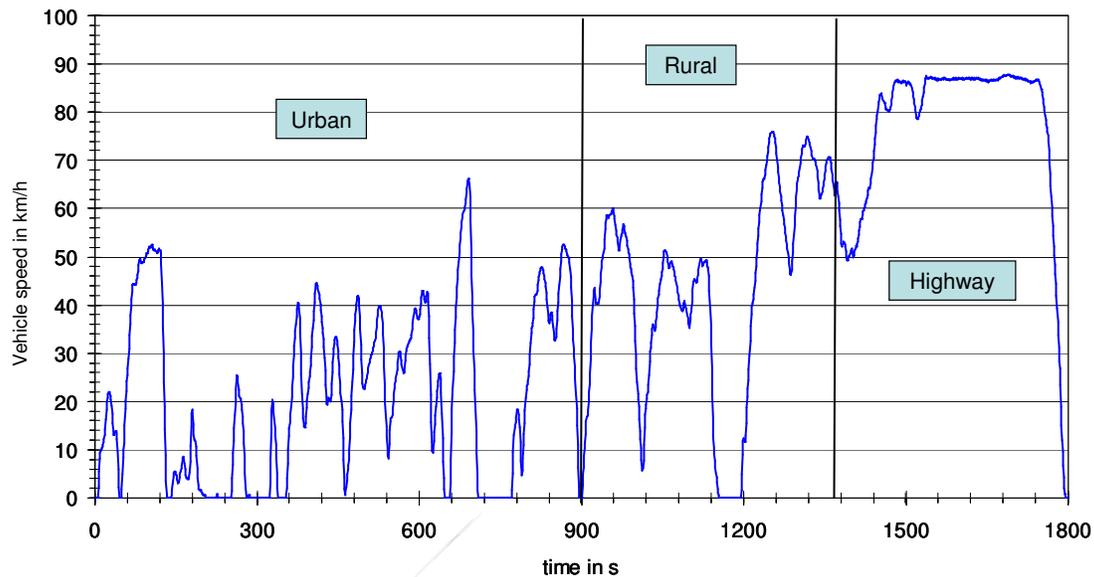
Figure 4 The WHVC test cycle
