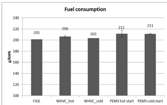
Figure 61 Brake specific fuel consumption.
