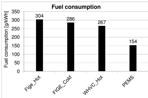
Figure 76 Brake specific fuel consumption.
