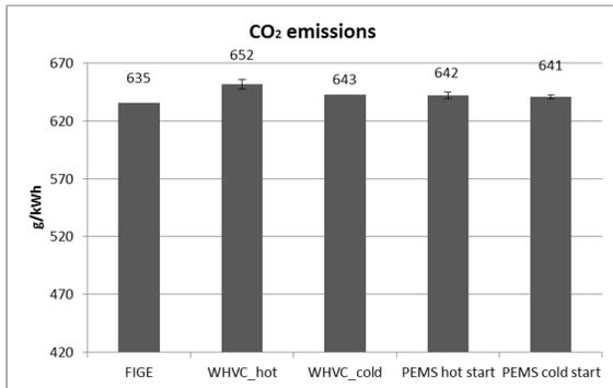
Figure 59 Brake specific CO<sub>2</sub> emissions.
