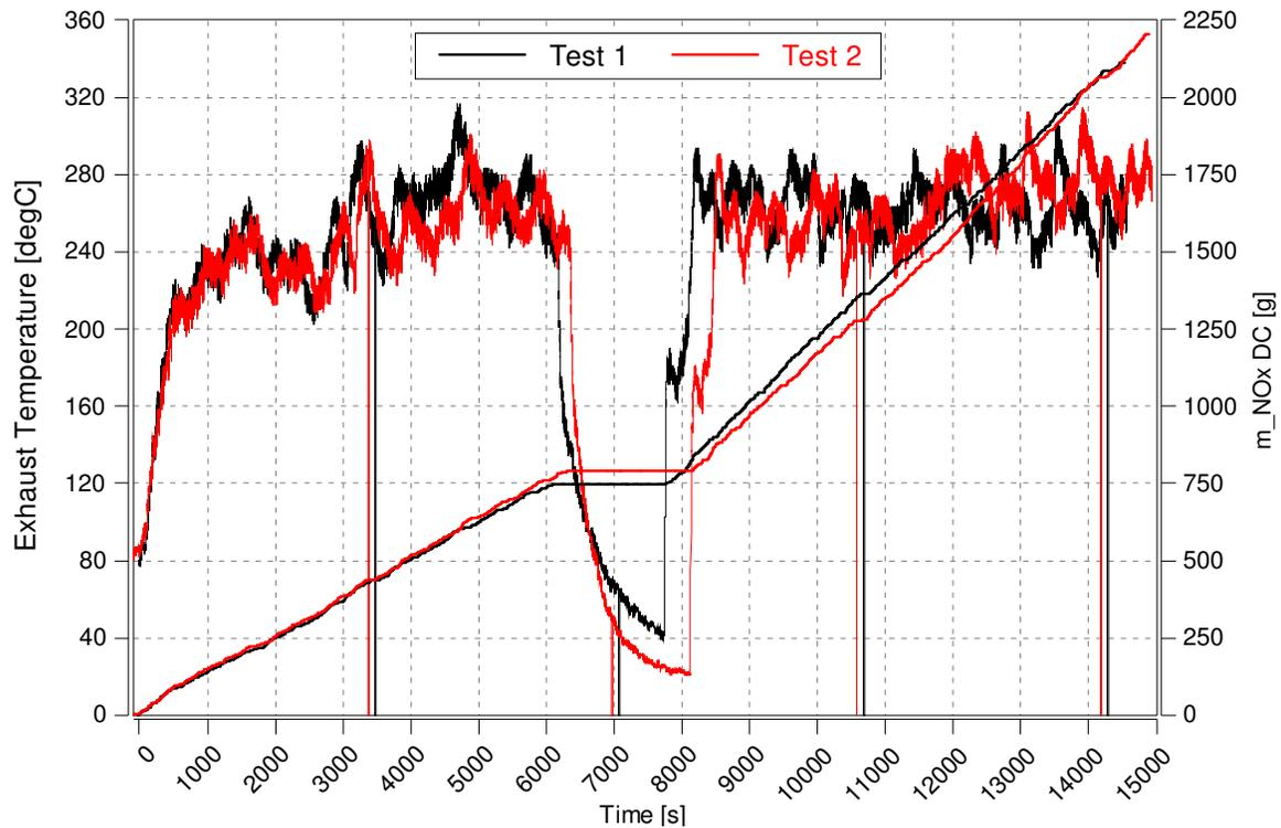
Figure 95 Tailpipe exhaust temperature and accumulated NO<sub>x</sub> during test 1 and 2 on the Euro VI route2.
