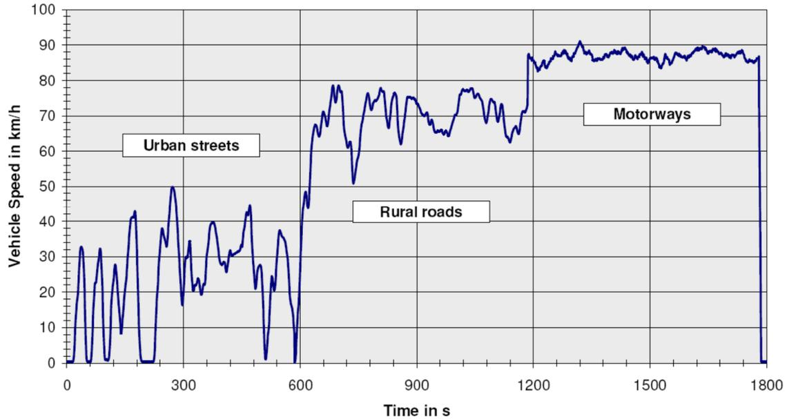
Figure 3 The FIGE driving cycle
