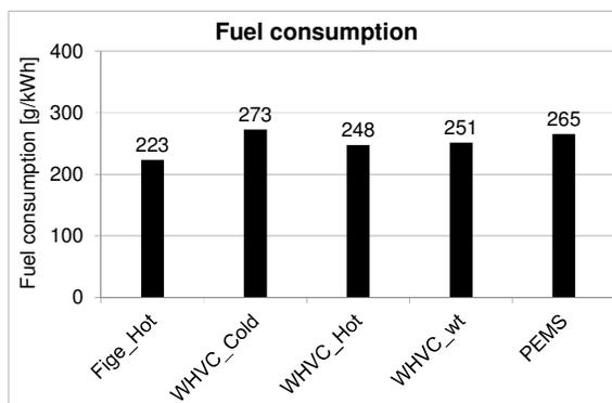
Figure 109 Brake specific fuel consumption
