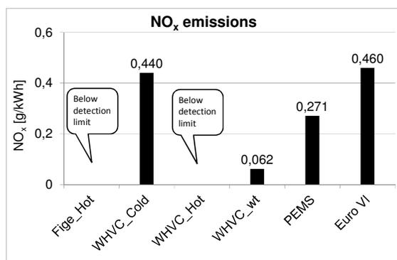
Figure 101 Brake specific NO<sub>x</sub> emissions.
