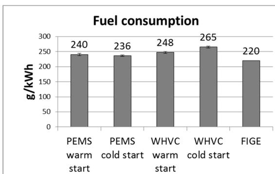
Figure 46 Brake specific fuel consumption.
