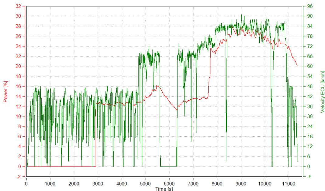
Figure 49 Engine power during one PEMS test
