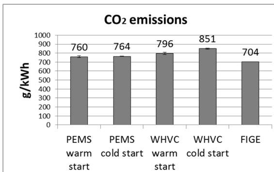
Figure 44 Brake specific CO<sub>2</sub> emissions.
