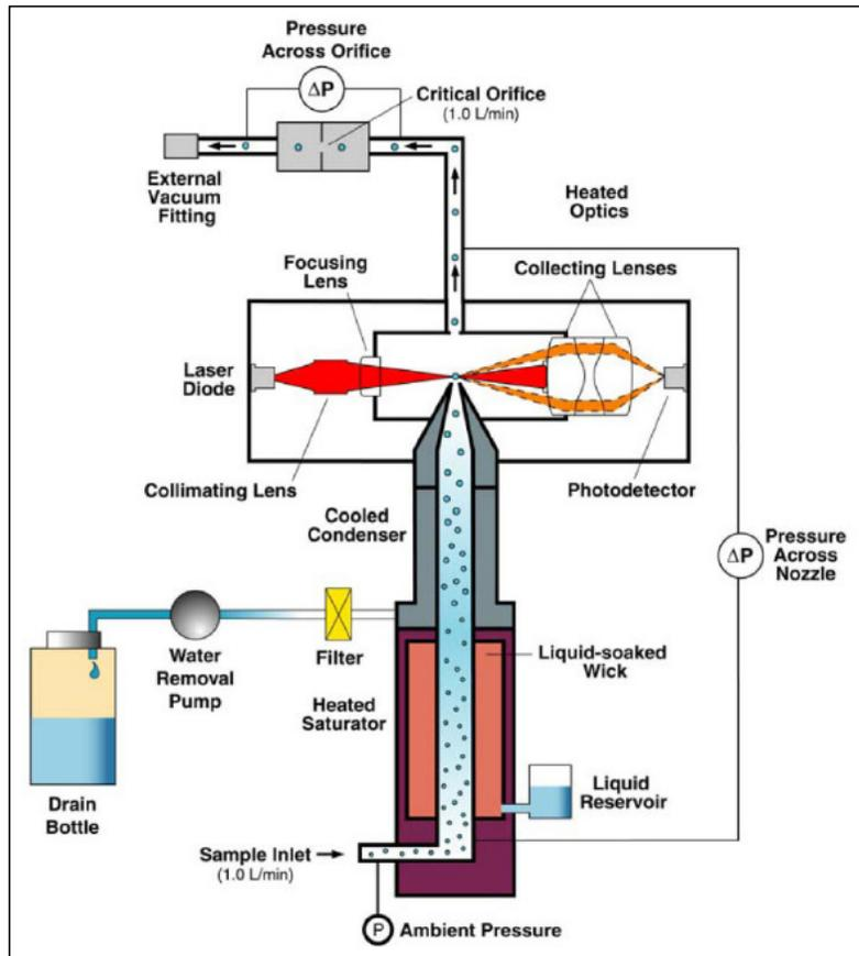
Figure 2 Schematic description of the detector in the Condensation Particle Counter.
