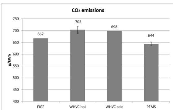
Figure 26 Brake specific CO<sub>2</sub> emissions.
