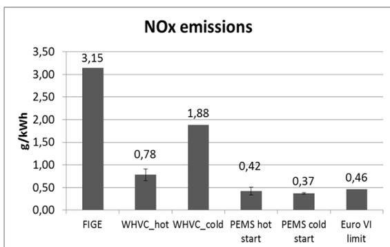
Figure 55 Brake specific NO<sub>x</sub> emissions.
