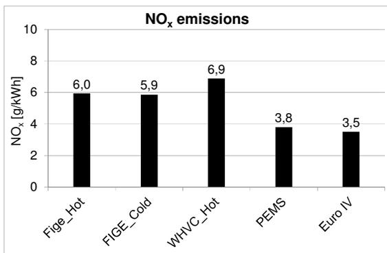
Figure 68 Brake specific NO<sub>x</sub> emissions.
