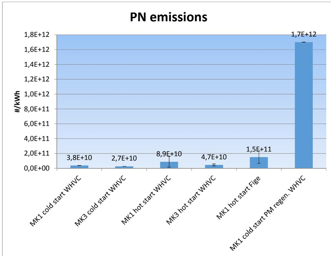
Figure 123 Particle number emissions g/kWh.
