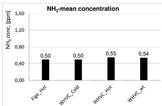
Figure 112  $\text{NH}_3$  test cycle mean concentration in exhaust gas.
