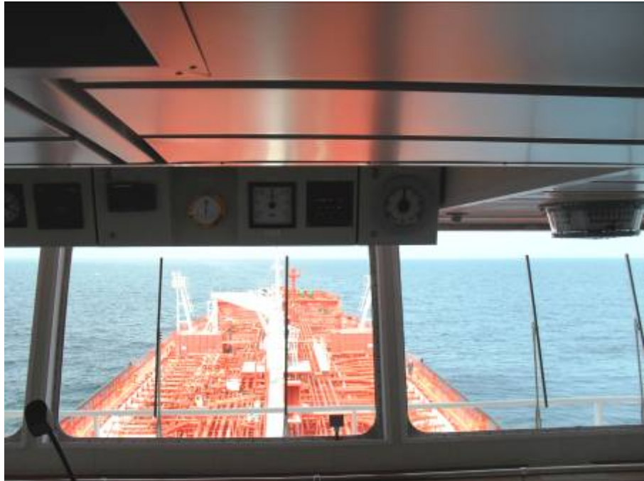
Picture 11 – View over the front edge of the bridge with the indicators showing rudder position and turning rate.
