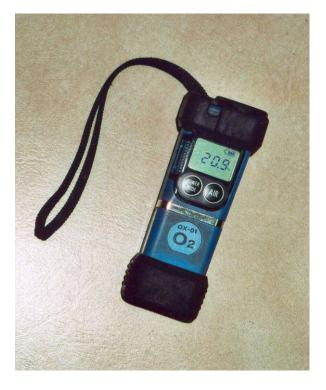
According to the safety manual an oxygen meter shall be used and be carried by the person who intends to enter an enclosed space.
