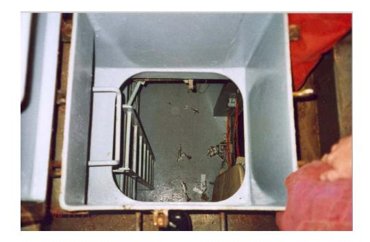
From the first platform there was a steep staircase, which also ended at a platform with a similar door to the hold. Yet another steep staircase ended on the tanktop with a door which led to the bottom of the cargo hold and which also opened to the trunk (see sketch page 7).
