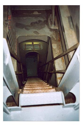
The function of the two upper doors was to give access to the cargo hold at different levels of cargo. From the access opening on weather-deck it was not possible to see the lower entrance to the cargo hold since the platforms and the staircases blocked the view.
