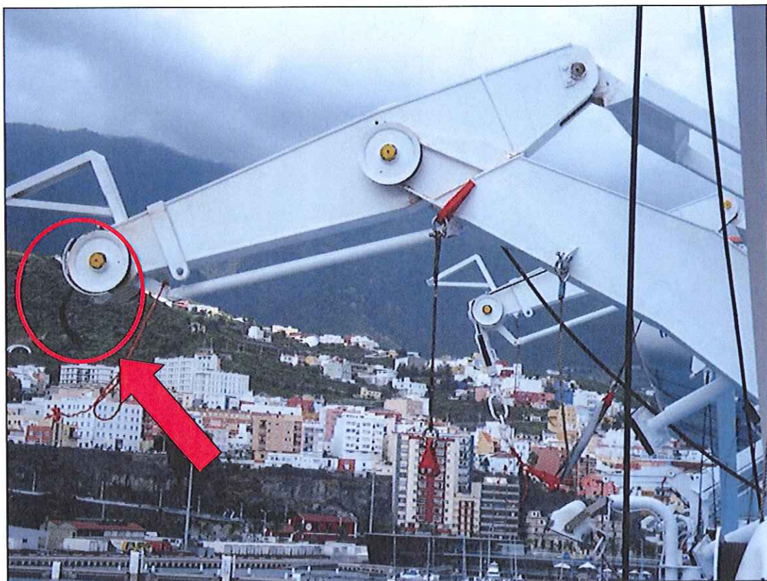
Forward Davit Arm Showing Parted Wire
