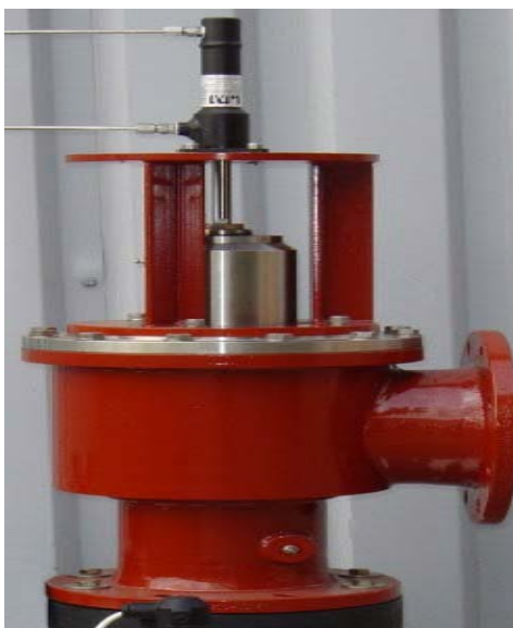
Figure 4.1 – Hydraulically controlled VOCON valve
