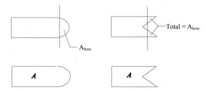
Figure 4.4.1: Plan view of two different craft styles
