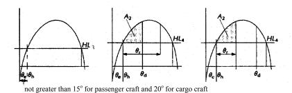
Figure 2 - Damage stability
