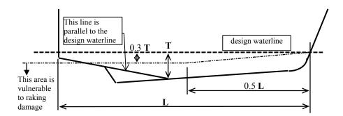
where: T = maximum draught of the hull (each hull considered individually in the case of multihulls) to the design waterline, excluding any non-buoyant structure, provided that structures such as single plate skegs or solid metal appendages shall be considered to be non-buoyant and thus excluded.<sup>22</sup>
