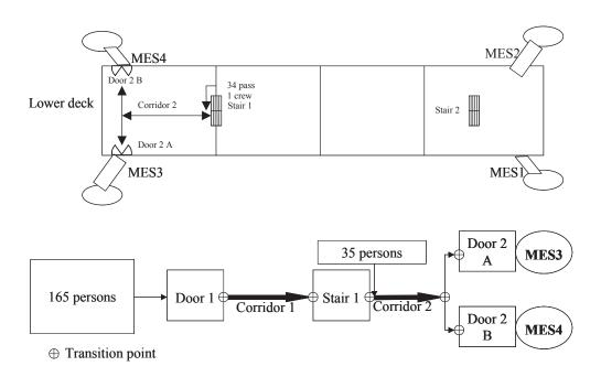
Figure 4 – Sketch of the evacuation path and its schematization
