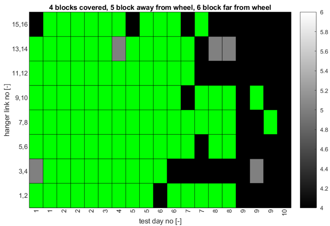
Figure 62 Ice build-up on blocks and holders for tests with sinter blocks on wagon 5.
