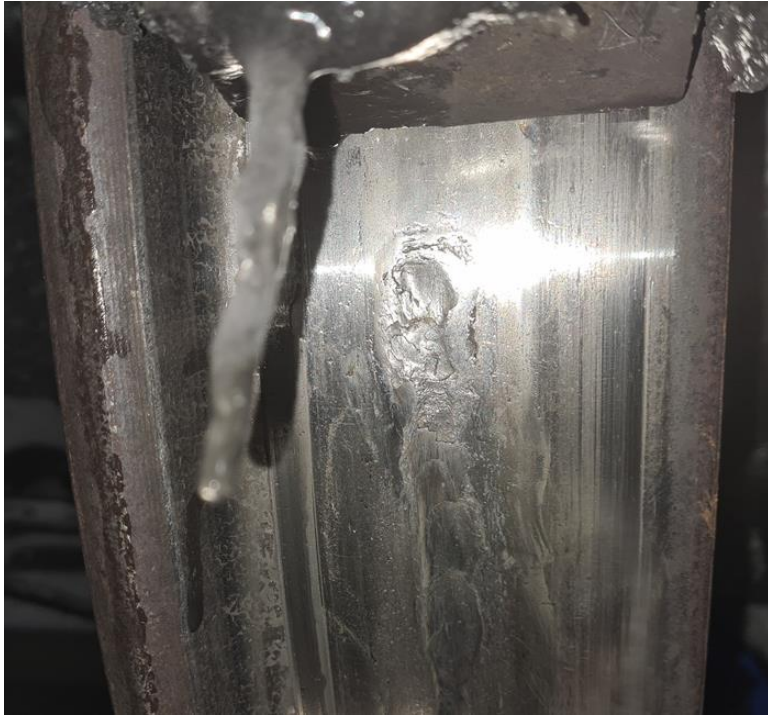
Figure 10 Example of wheel tread damage resulting from braking with loaded wagons. In top of picture is lower part of block with an icicle.
