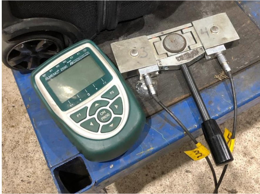
Figure 71 Photo of data logger and one of the two force transducers that was mounted between blocks and wheel.
