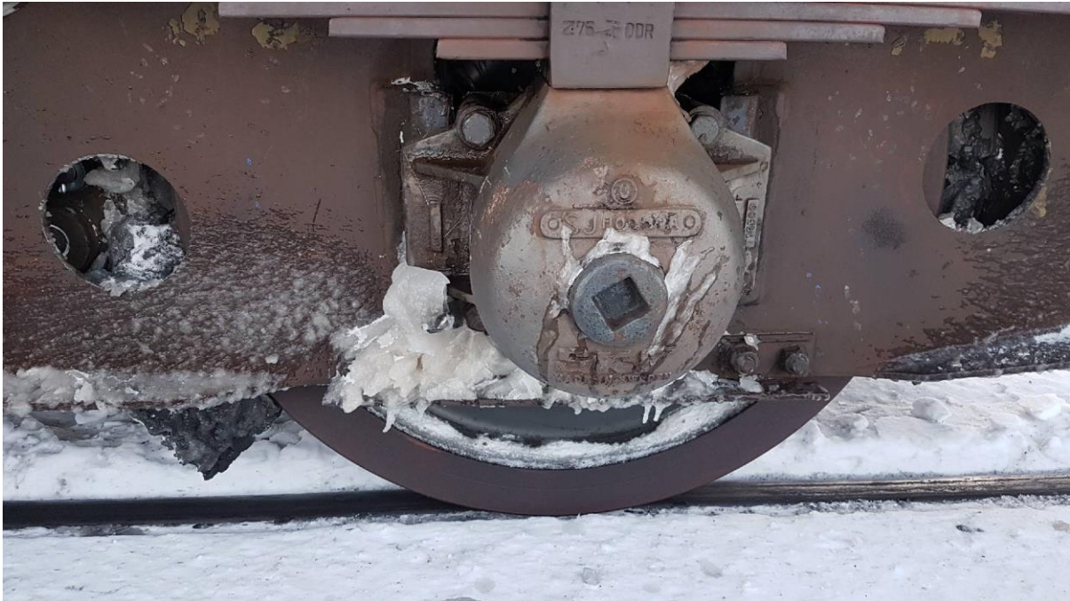
Figure 18: Photo of ice build-up on trailing brake shoe. The vehicle has been running in right direction before photo is taken.
