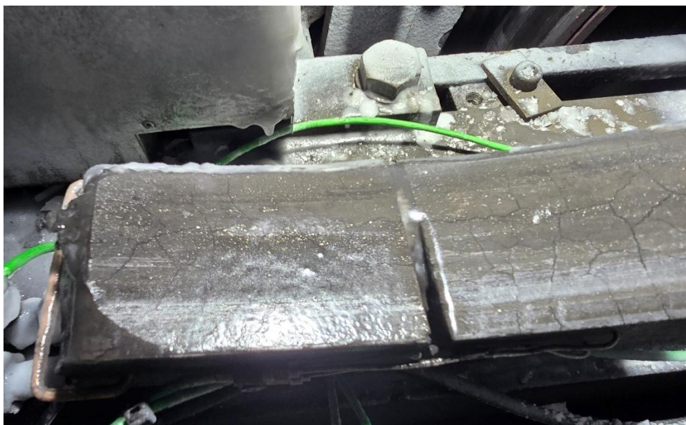
Figure 4. Brake block J822 with a thin layer of ice on the friction surface
