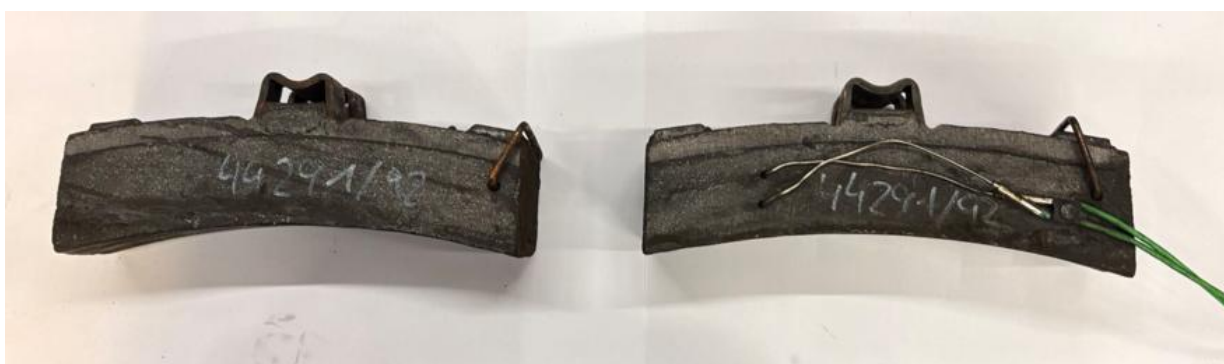
Figure 2. Photos of brake blocks: J822 (top) and C333 (bottom), with embedded thermocouples in one brake block, and a small handle to be able to easily mount and dismount the brake block. Photos are taken after the tests.
