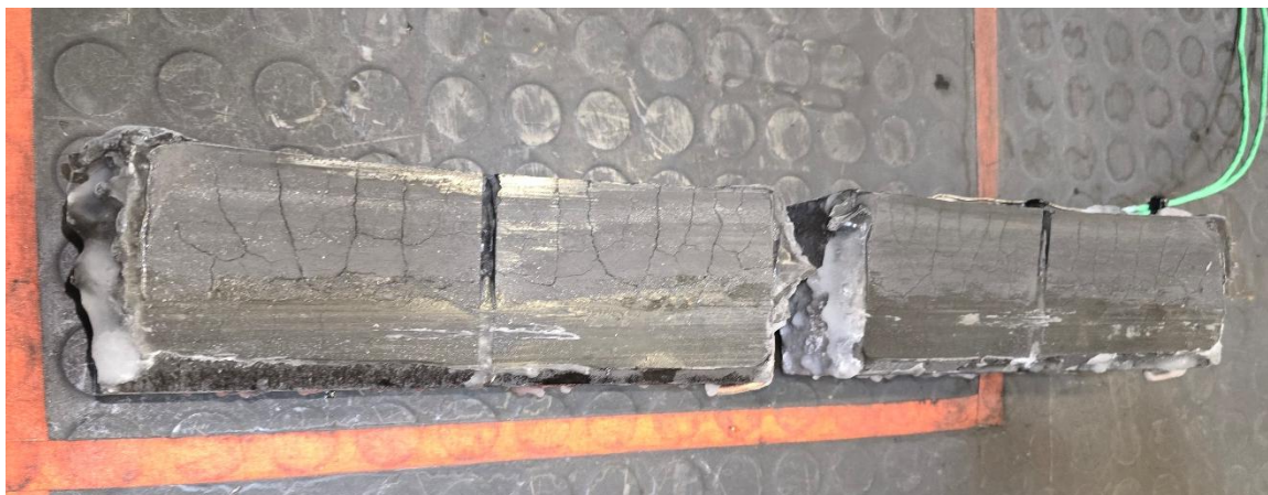
Figure 8. Brake blocks with remaining ice on friction surface. After brake cycle no 6, with 7,5 kN, and after conditioning brake from 50 km/h. Picture is taken directly after the brake blocks are removed from test bench.
