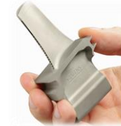
Turbine blade printed & tested in engine (SGT-100)
