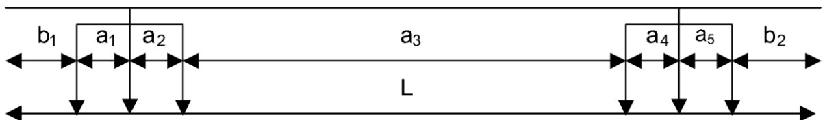
Figure 1: Longitudinal vehicle dimensions
