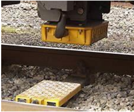
Example 1: Automatic Train Protection system
