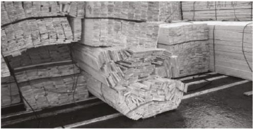
Figure 6.2. Example of poor rigidity
