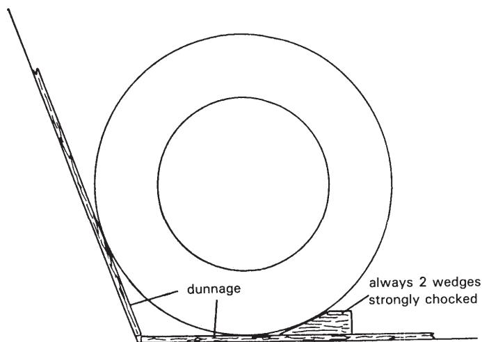
Figure 1 – Principle of dunnaging and wedging coils
