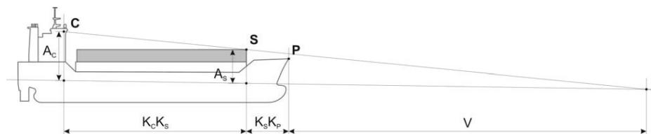
**Figure 3.1. Distances used for calculating the bridge visibility**
