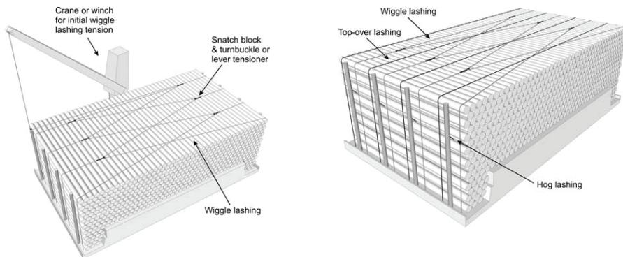
**Figure 2.3. Example of wiggle lashings**
