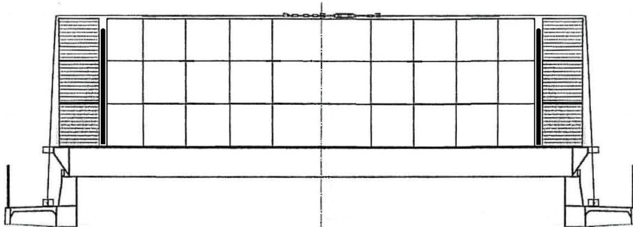
**Figure 6.4. Sliding of upper layer prevented by vertical sturdy battens**
