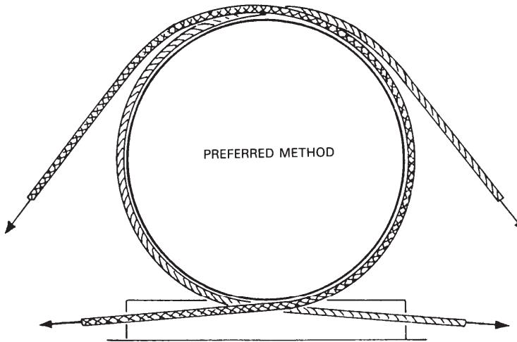
Figure 1 – Securing of receptacles having no securing points
