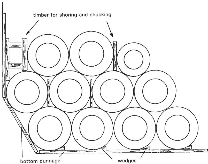
Figure 3 – Shoring and chocking in voids between coils
