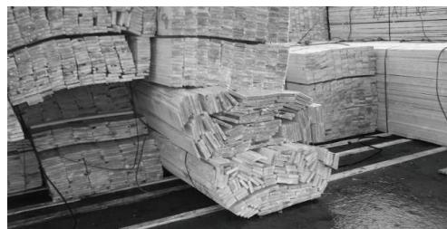
**Figure 6.2. Example of poor rigidity**
