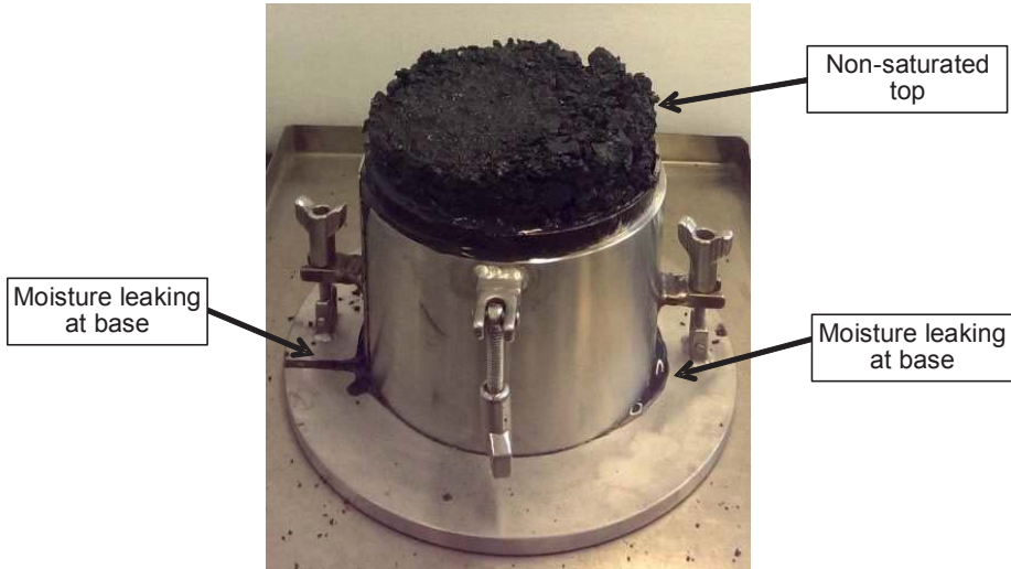
Figure 1.5.8 Test showing water leakage from the base of the cylindrical mould indicating moisture migration
