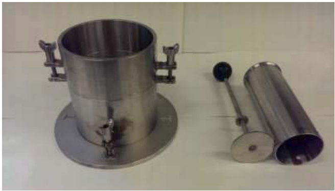
Figure 1.5.1 Example of Proctor/Fagerberg test apparatus, hammer and hammer guide
