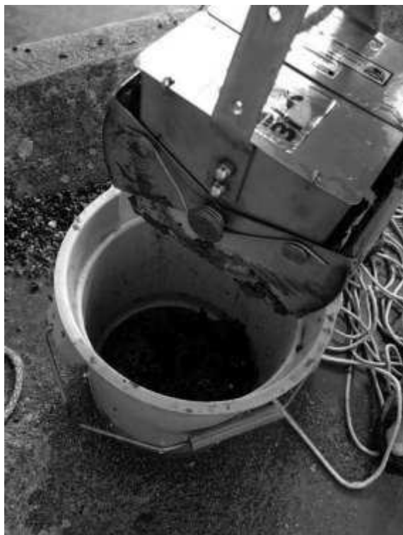
Figure 4. Benthic sample obtained by using an Ekman Grab.
